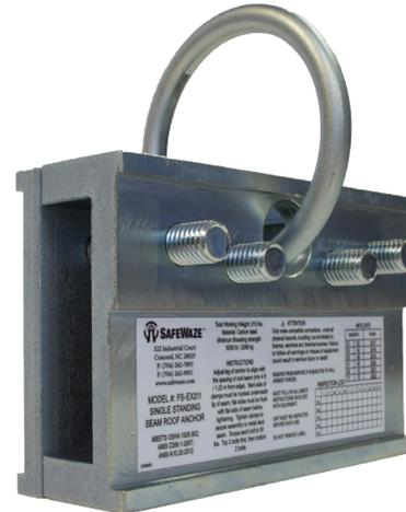
**Description** The Safewaze™ metal standing seam roof clamp is a rated roof anchor point designed for sloped or flat roofs. Must be rated to meet OSHA, federal, state and local government regulations for fall protection anchor points. MINIMUM required substrate thickness: 24 gauge
